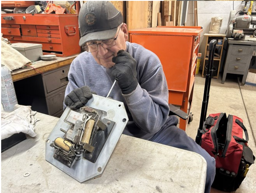
Lee repairs bell ringer for PAT Transit 1713 aka The Terrible Trolley. Scott Becker photo
