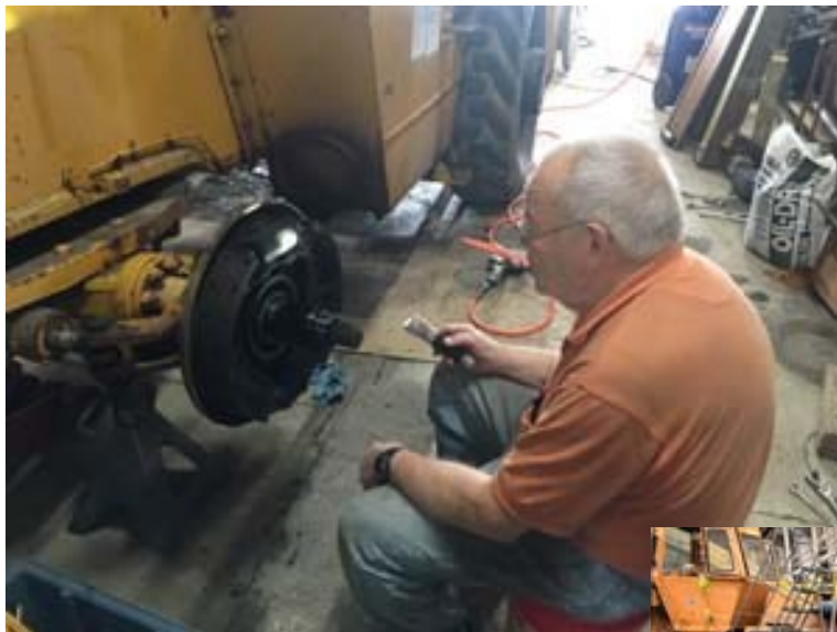
Dave Hamley works on replacing the Galion Crane's rear brakes. Scott Becker photo
