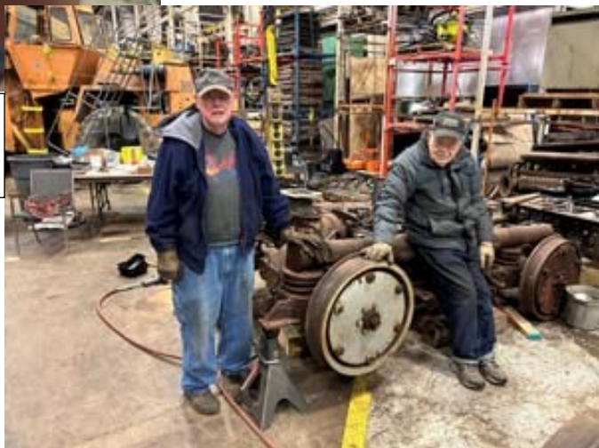
Dick Rhoton and Dave Hamley have successfully test fitted Shaker Heights wheels using a Pittsburgh Railways axle. 4-3-24 Scott Becker photo
