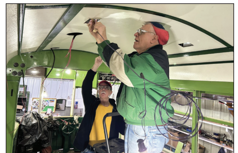
Barrie Baker and John Habak work on 8042's interior lights. Scott Becker photo
