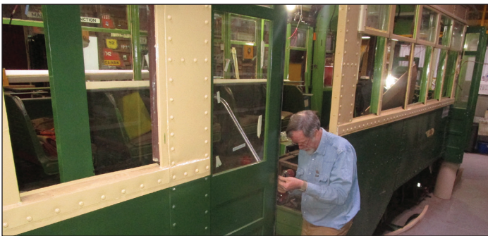
Scott Becker captured Keith Bray installing center doors on Philadelphia Transportation Co. 8042.
