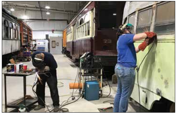
Our "Cleveland Crew" has been hard at work sanding, cleaning and priming in preparation to repaint Shaker Heights 94. Following the first day of sanding, Kevin Zebley spearheaded the effort to weld patches in the rust holes in the car, assisted by Laura Wells.
