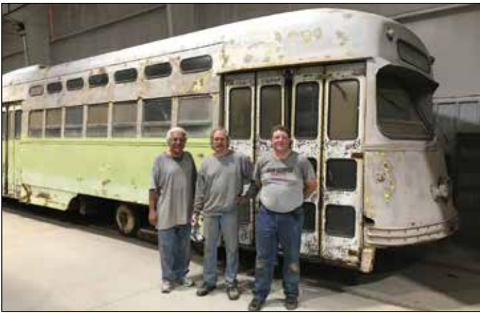
Our "Cleveland Crew" has been hard at work sanding, cleaning and priming in preparation to repaint Shaker Heights 94. Following the first day of sanding, Kevin Zebley spearheaded the effort to weld patches in the rust holes in the car, assisted by Laura Wells.
