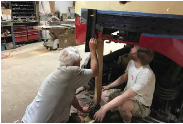
Eric Weinbrenner and Brett Freithaler put pressure on the skirt of 1138 in an effort to straighten it. Photo by Bruce Wells
