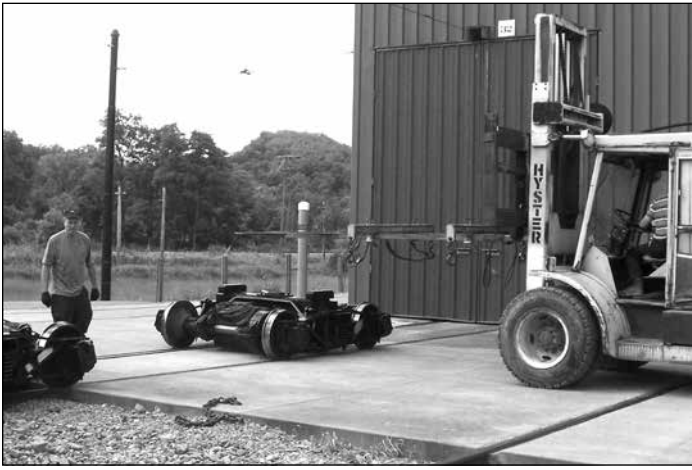
Bernie Orient and Larry Lovejoy unloading the rebuilt trucks for M283 and a close up of the finished product.
