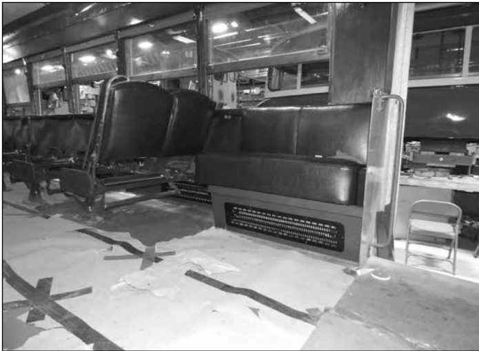
Rebuilt seat frames, new sandbox seats, reupholstered cushions new flooring and beautifully finished woodwork make are all pieces in the first class restoration of West Penn 832.
