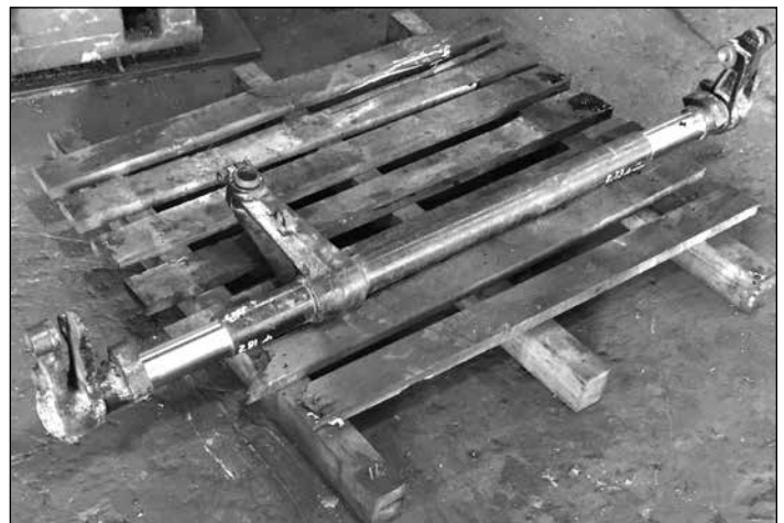
Rebuilt tread brake beams for Pittsburgh Railways 1138.
