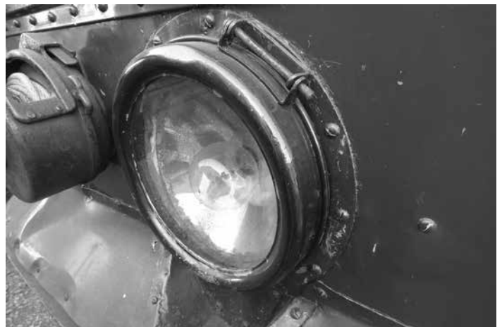
Original headlights for car 78 as found on car 80 at the Electric City Trolley Museum in Scranton
