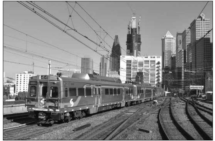
Silverliner V trains like this one were sidelined during the summer to repair cracked truck frames. Photo by Bill Monaghan
