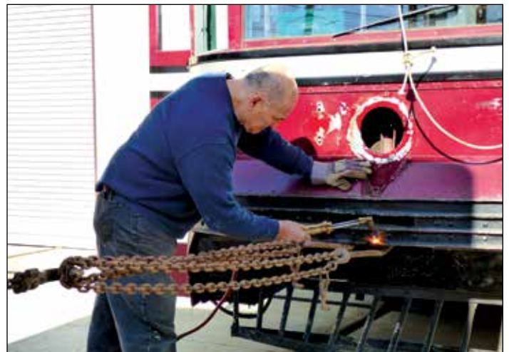
Ron heats 78's anticlimber while we were straightening it.
