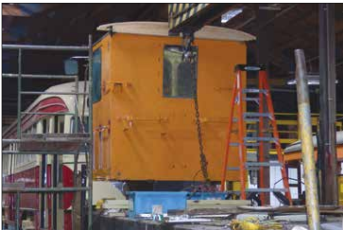
Crane Car M283 receives a new cab roof as part of the current rebuilding work underway in the shop.
